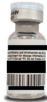
Figure 11. Barcode wraps around the curvature of the vial, not allowing it to be captured by a barcode scanner.
